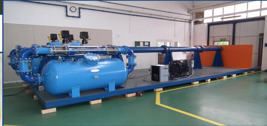
Pneumatic gun for impact tests in aviation
